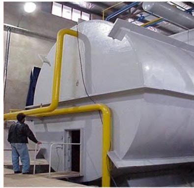
Photographs that Israeli officials said were stolen from Iran's nuclear archive appear to show a metal chamber constructed to conduct high-explosive experiments.
